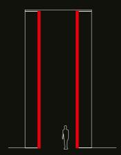
A massive sliding bronze door separates the light-flooded, shared lobby of two Sydney office towers. It is ten metres high, five metres wide and weighs a massive five tonnes. Opening or closing it by hand is not an option, so the sliding door must run automatically. Apart from its aesthetic appearance, it also fulfils a purpose: in an emergency, it serves as a fire door.
