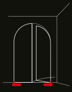
Filigree swing doors made of glass or massive doors in historical buildings are difficult to automate without visible drive technology. By the same token, the usual lintel-mounted drives are not an option for doors with round arches or other shapes. Monument preservation orders may also pose challenges for door automation. For all these situations, TORMAX offers the appropriate, invisible drive solution which is fully recessed in the floor or in the door lintel.
